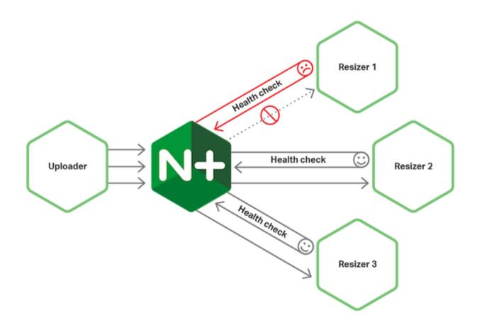
Prevent cascading failures by using a circuit breaker that can temporarily stop requests to a failing service and provide fallback mechanisms.
