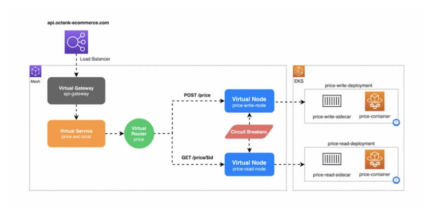
Isolate failures within separate sections to prevent them from affecting the entire system.
