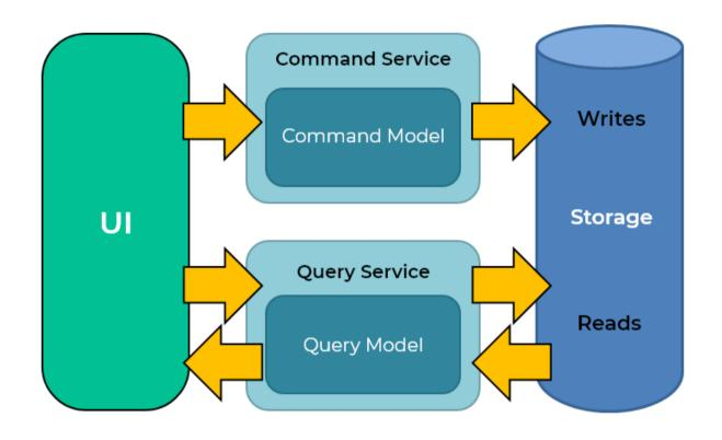
Separate the read and write responsibilities of a system, allowing for optimized performance and scalability.
