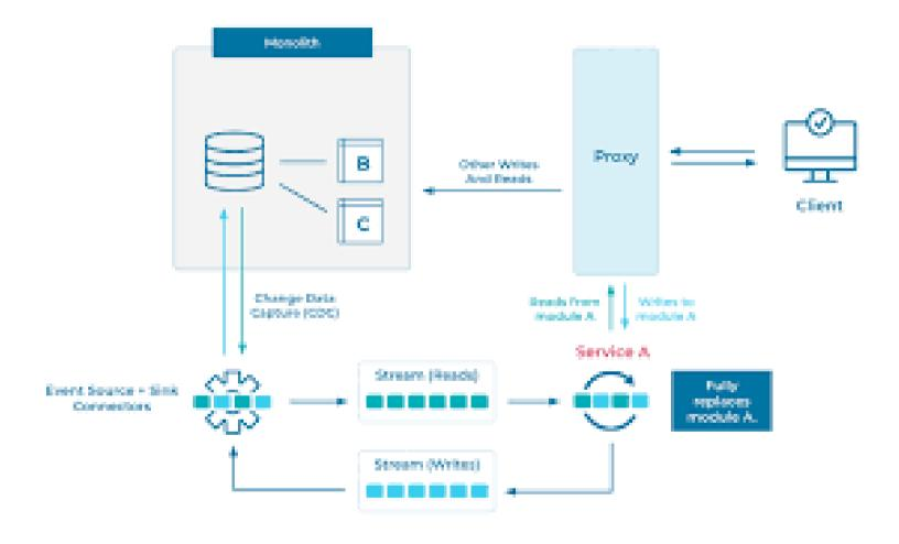
Gradually replace components of a legacy system with new ones until the old system is "strangled" and replaced entirely.
