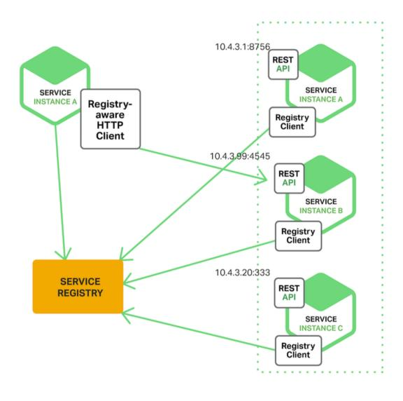
Implement a service registry to automatically locate and register microservices. This helps in dynamic discovery and communication between services.
