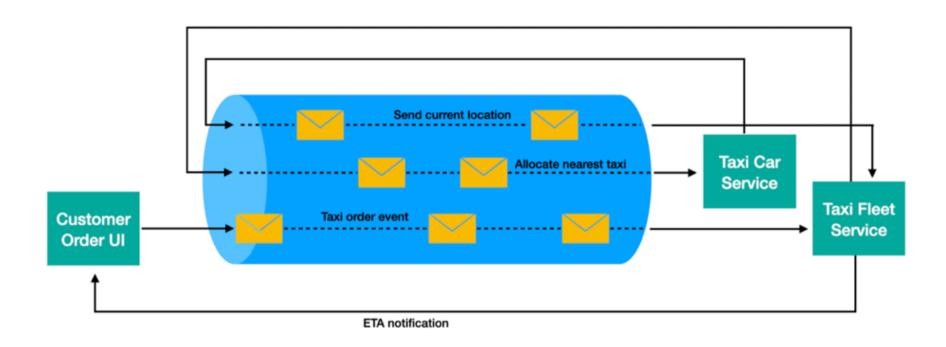
Communicate between microservices through events, enabling loose coupling and scalability.
