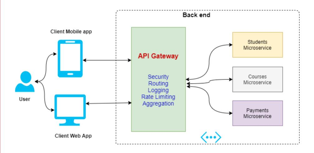
Use an API Gateway to handle client requests and route them to the appropriate microservices. This centralized authentication, load balancing, and routing logic.
