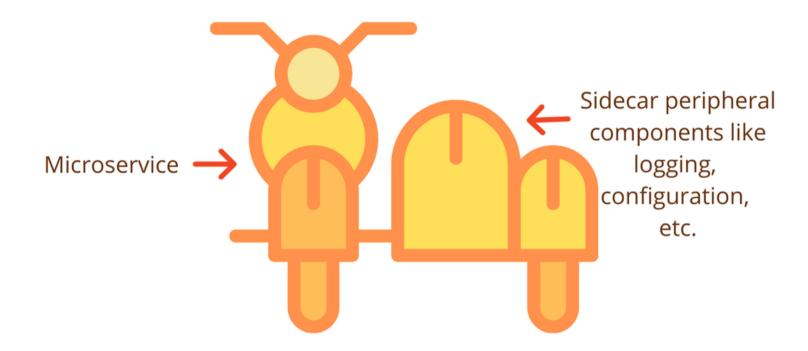
Attach a separate microservice (sidecar) to handle specific tasks like monitoring, logging, or authentication.
